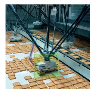
Choosing the right rejection mechanism (air jet with nozzles, independent traps, retractable belts, robot, etc.) is important to ensure non-compliant products are accurately removed from the production line. To determine the most suitable option, it is important to consider several factors, such as: type and dimensions of product, how they are presented into the vision inspection system, line width (up to 5m) and speed, space available, etc.
