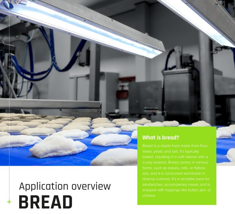
With SENSURE SYNAPSE, it is possible to **measure numerous product features** (a wide set is included in the system), such as shape, size, and colour, using **2D technologies** (industrial cameras) and perform a full 3D product profile using **3D technology** (laser profilometer). SENSURE solutions also allow for the inspection of the bottom part of products.
